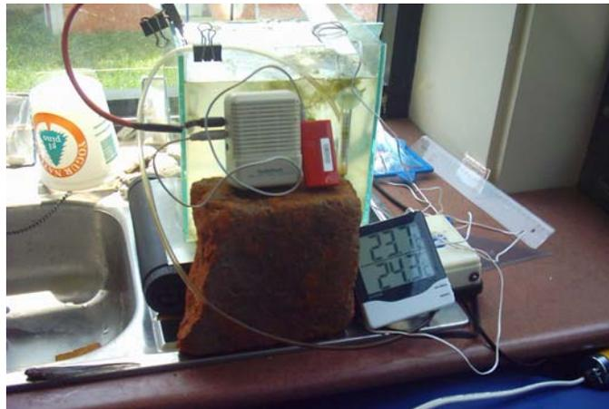
*Our experimental set up includes an aquarium with 7 l water. We adjusted the water conductivity around 2000 microsiemens, measured the temperature during experimentation by a thermometer with an electronic display. Eigenmannias EOD signals were amplified with Radio Shack mini amplifiers and recording done with CREATIVE, Panasonic audio devices. Changes of water temperature were established by a small kitchen cooking devices below the aquarium.*
